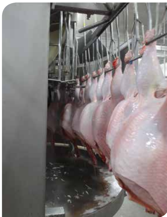
The use of in-process carcass sprays and inside/outside bird washers like the one shown here, can significantly impact the levels of bacteria on bird carcasses.
